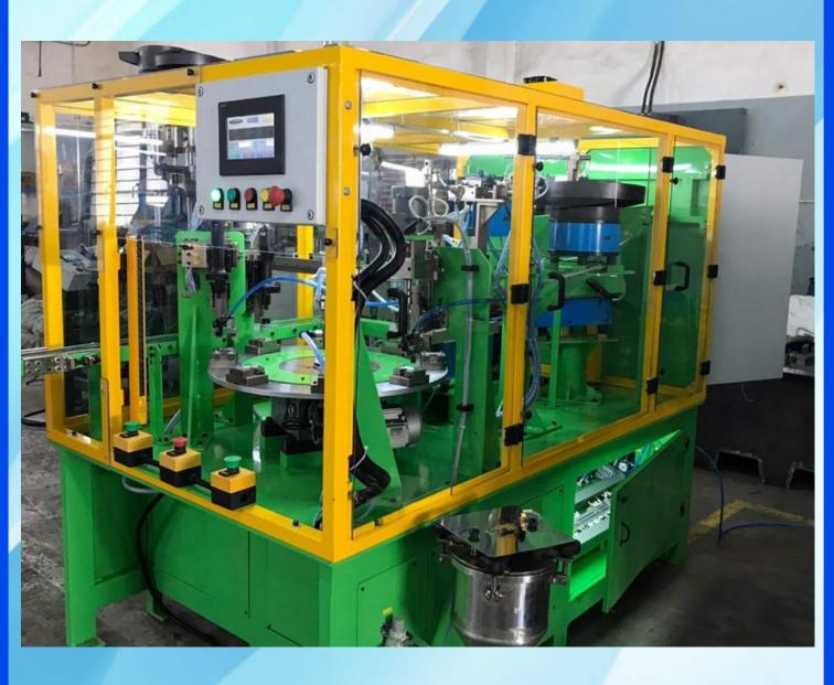
Heat sink assembly machine with I C
