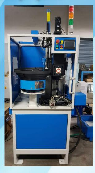
Automatic Nut Tapping Machine production capacity is 20 parts per minute.
