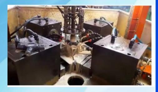
UJ Cross Servo Drilling Machine Cross 4-way Drilling Machine
