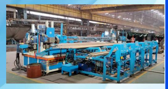
Circular Saw cutting machine to Cut Steel bars Dia 20mm to 160mm
