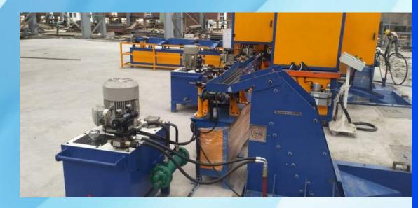
Billet chamfering Machine chamfers the Billet both corners with cycle time < 7 to 10 sec
